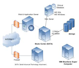
Fig. 1. Information technology structure for the THEW. Two options are proposed to access the data from the THEW: 1) Server hosted at University of Buffalo based using secured file transfer protocol (SFTP), 2) THEW client application which is a dotNET client server application providing the access to both ECG signals and the associated clinical information.
